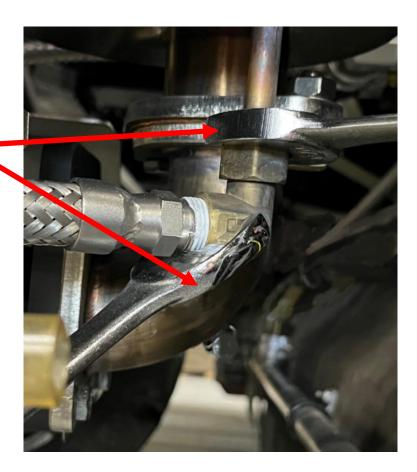
Use a 7/8 and 13/16 wrench to remove fitting from heat exchanger:
