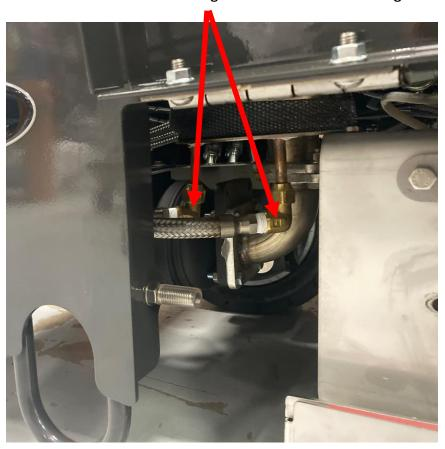
Make sure to secure both the flare nut on the heat exchanger and the brass fitting with with wrenches when loosening to prevent damage to the components.
